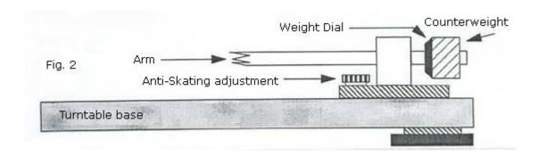
If the needle is not skipping in the groove, resist the temptation to crank up the tracking force greater than recommended. If you are working in a club with very bassy speakers, you may need to increase the weight a little to stop the needle from skipping. You can crank most Ortofon cartridges up to 5 grams if you need to.
