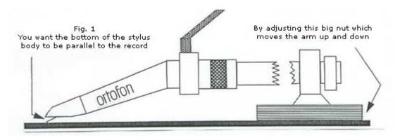
**Align the cartridge** in the slots in the headshell, if you are using a standard 1/2" mount cartridge. Use the alignment card supplied with the turntable if available. If you don't have one, place the cartridge half way up the two slots in the headshell. If you are using an Ortofon Concorde then no alignment is required as it screws straight into the arm.
